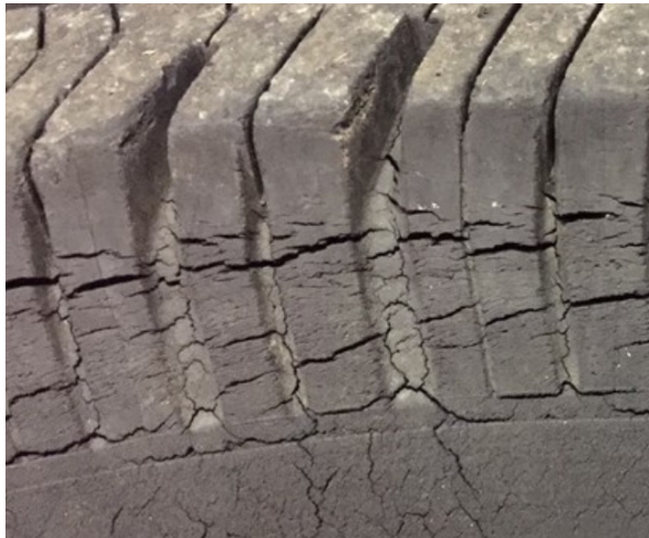
Tire Rubber Cracking
